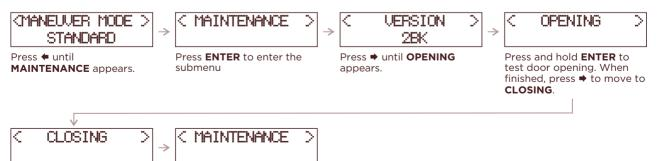
Press and hold **ENTER** to test door closing. Close the door completely. Press **BACK** to exit the submenu. **7** Perform the maneuver programming procedure. Make sure you have closed the door first.
